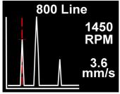
The Vib Meter 330 includes a high resolution zoomable vibration spectrum display with fully dynamic cursor displaying frequency and amplitude values.
